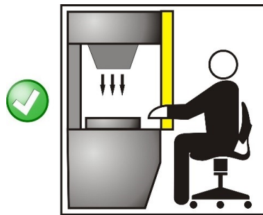
Figure 6: Correct light curtain positioning
